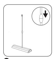
Assemble the two piece pole, and insert the round end in the base.
