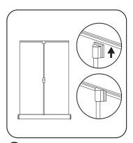
Tilt the top bar back on a slight angle to position the fitting at the top of the pole into the channel in the center of the top bar.
