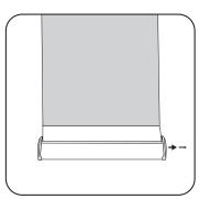
Gripping the banner securely with one hand, remove the locking pin from the right side of the base.
