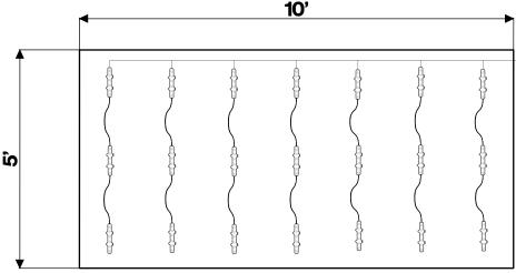
Load: 75.6 Modules: 21 Watts: 113.4 of 150.0 PS: HanleyLED 150w 24v
