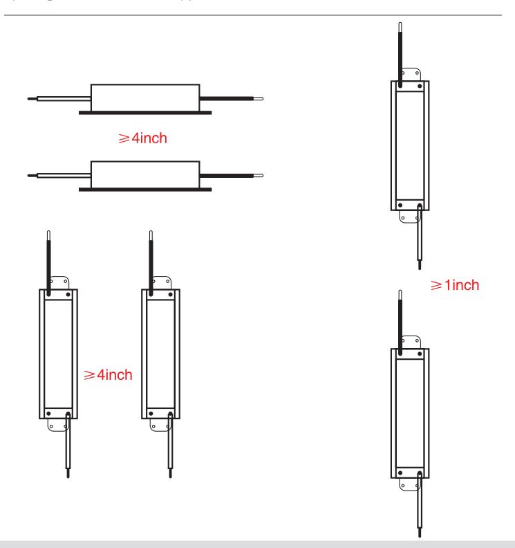
UL 48 Standard requires spacing between LED power supplies shall be at least 1 inch from end to end and 4 inches from side to side. This is to ensure adequate heat dissipation. Greater spacing may be required when heat ventilation in the sign or power supply enclosure is not adequate.
